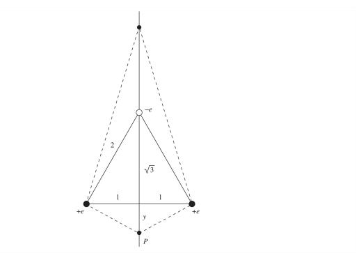
If the electric field equals zero at *P*, then the upward field due to the negative ion must cancel the downward field due to the two positive ions. This gives
